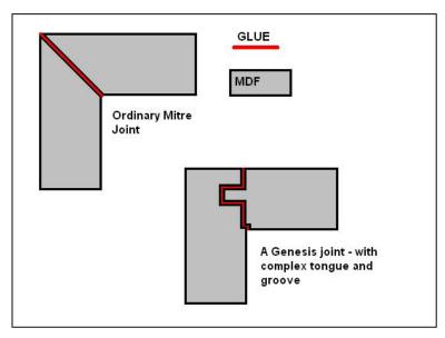
Genesis designed a unique tongue and groove joint in order to improve the structural rigidity of the cabinet.
